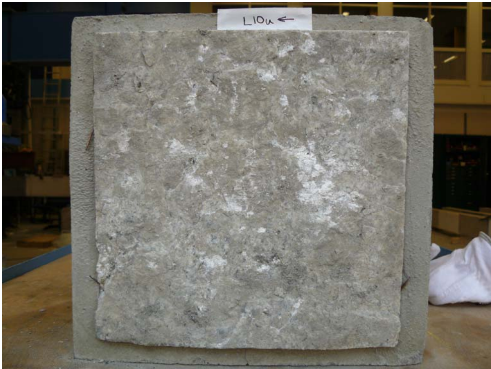
Picture B.14a Sample L10 after the shear test (lower part).
