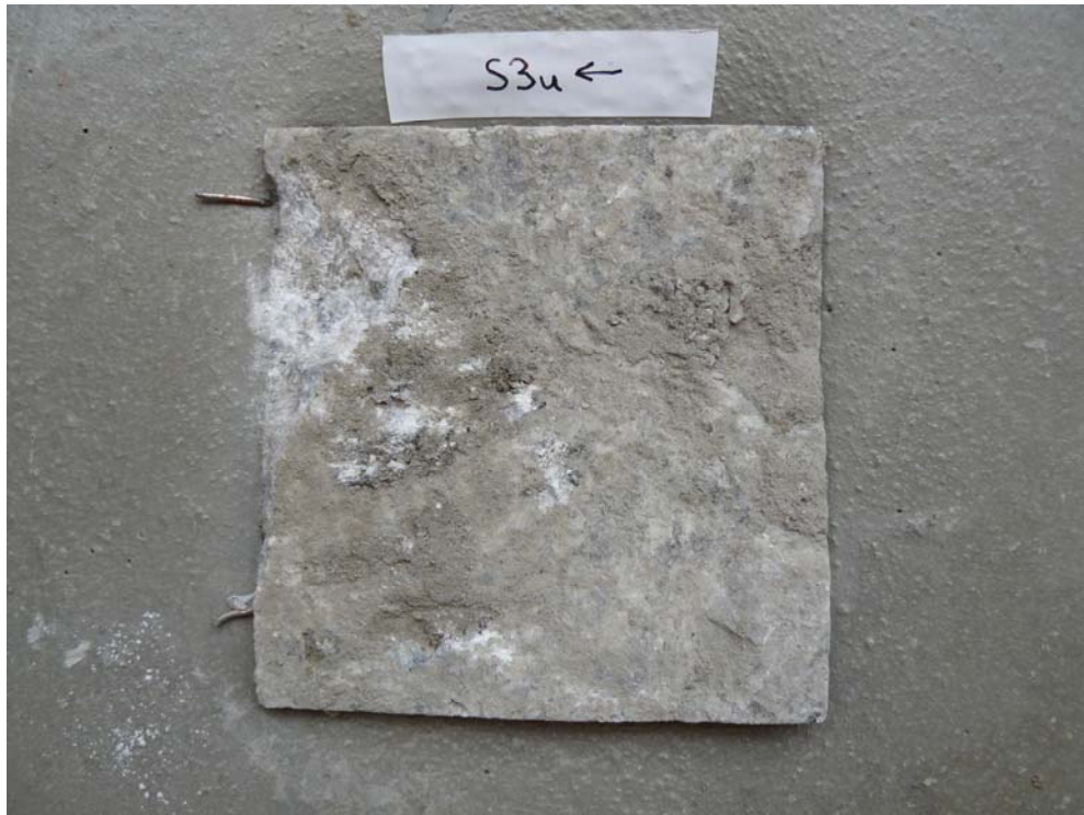
Picture B.3a Sample S3 after the shear test (lower part).
