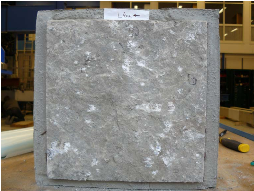
Picture B.10a Sample L6 after the shear test (lower part).
