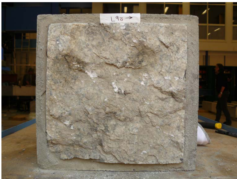
Picture B.13b Sample L9 after the shear test (upper part).
