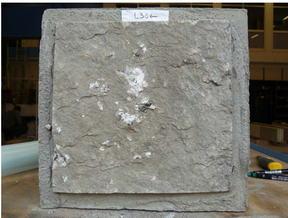
Picture B.8b Sample L3 after the shear test (upper part).
