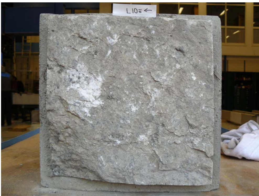
Picture B.14b Sample L10 after the shear test (upper part).
