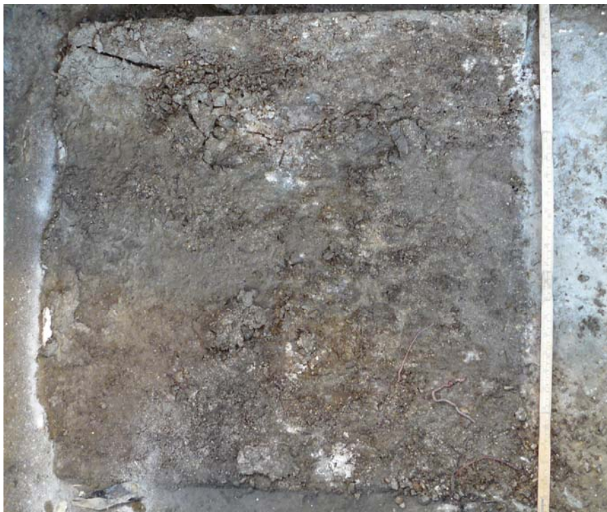
Figure 5.38 Lower part of the untouched joint surface after the upper block has been tilted.
