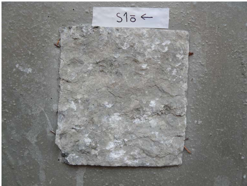
Picture B.1b Sample S1 after the shear test (upper part).
