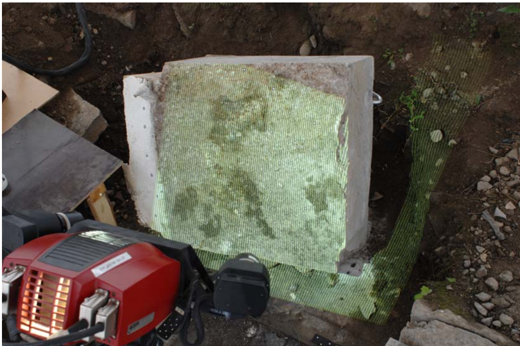
Figure 5.37 Measurement of surface roughness with optical scanning.
