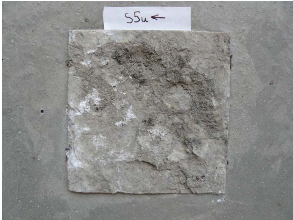
Picture B.5a Sample S5 after the shear test (lower part).
