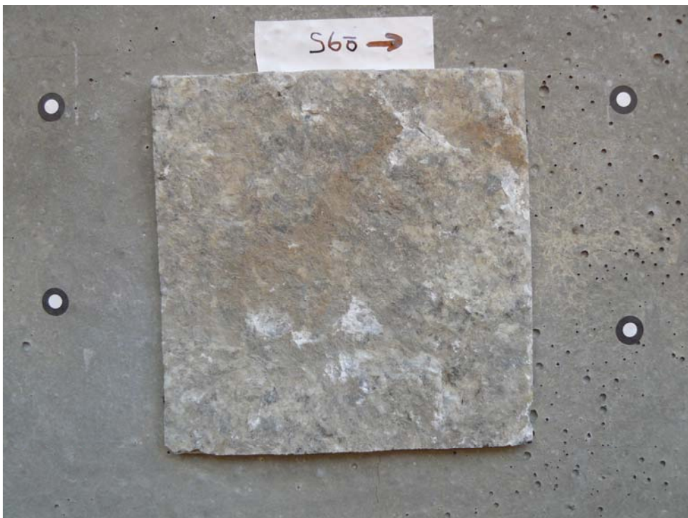
Picture B.6b Sample S6 after the shear test (upper part).
