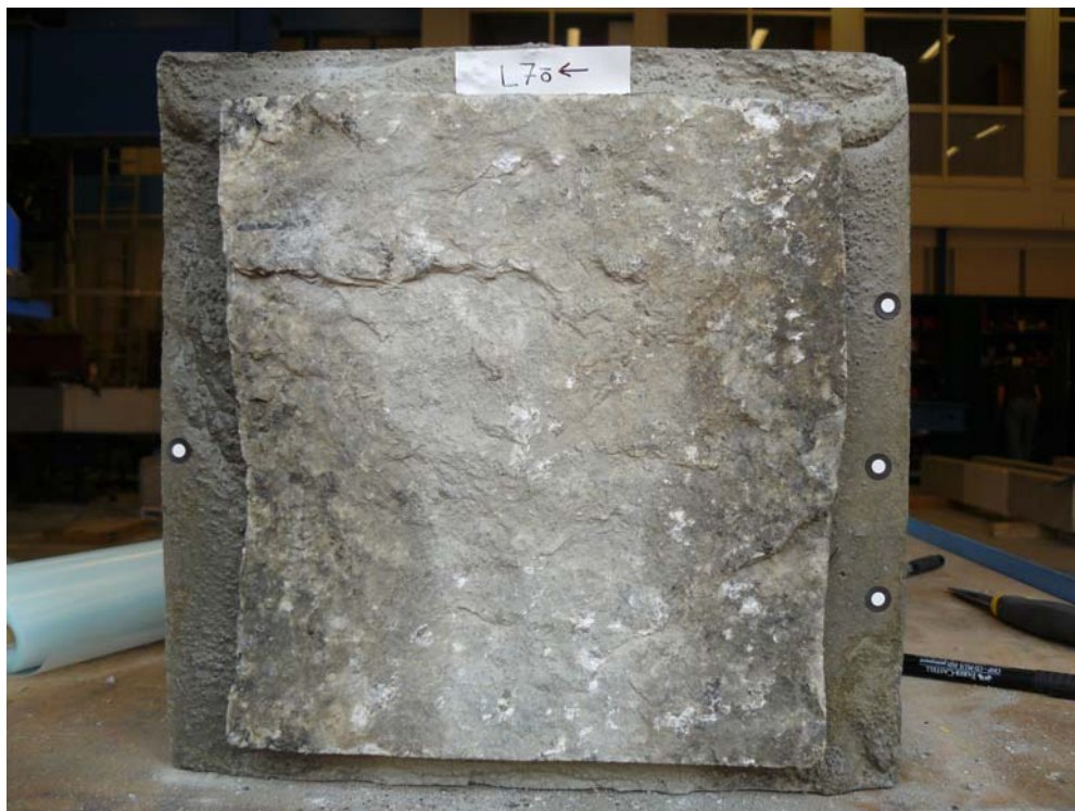
Picture B.11b Sample L7 after the shear test (upper part).
