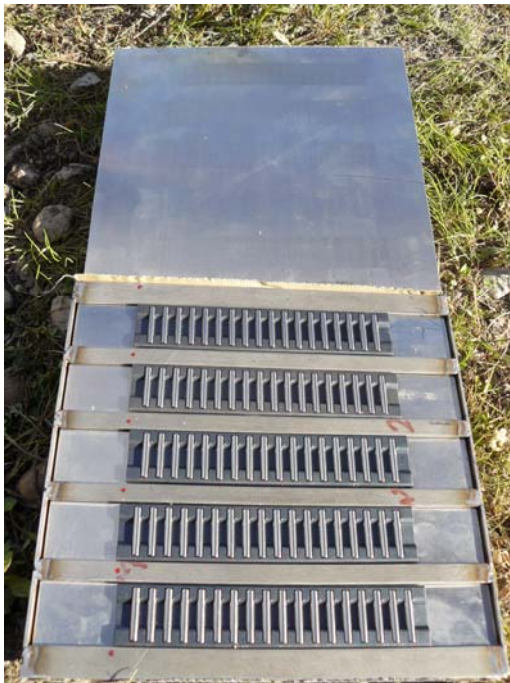
Figure 5.29 Sliding layer constructed by five flat roller cages and two 10 mm hardened steel plates.
