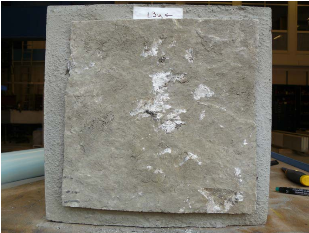
Picture B.8a Sample L3 after the shear test (lower part).
