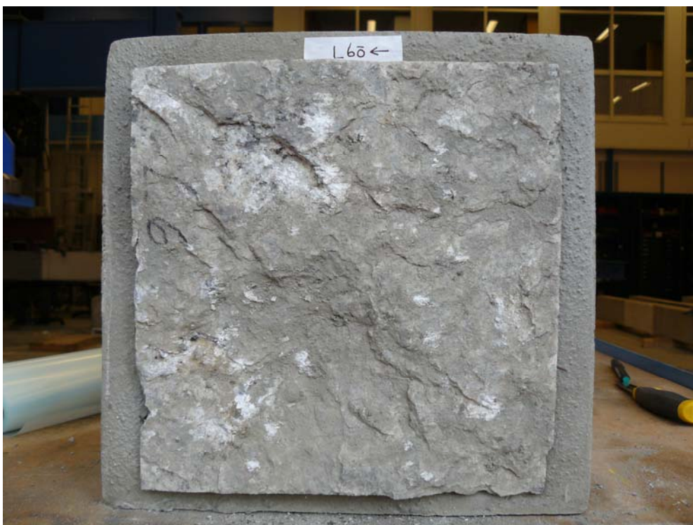
Picture B.10b Sample L6 after the shear test (upper part).
