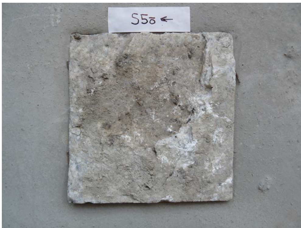
Picture B.5b Sample S5 after the shear test (upper part).
