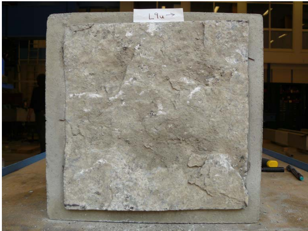
Picture B.13a Sample L9 after the shear test (lower part).
