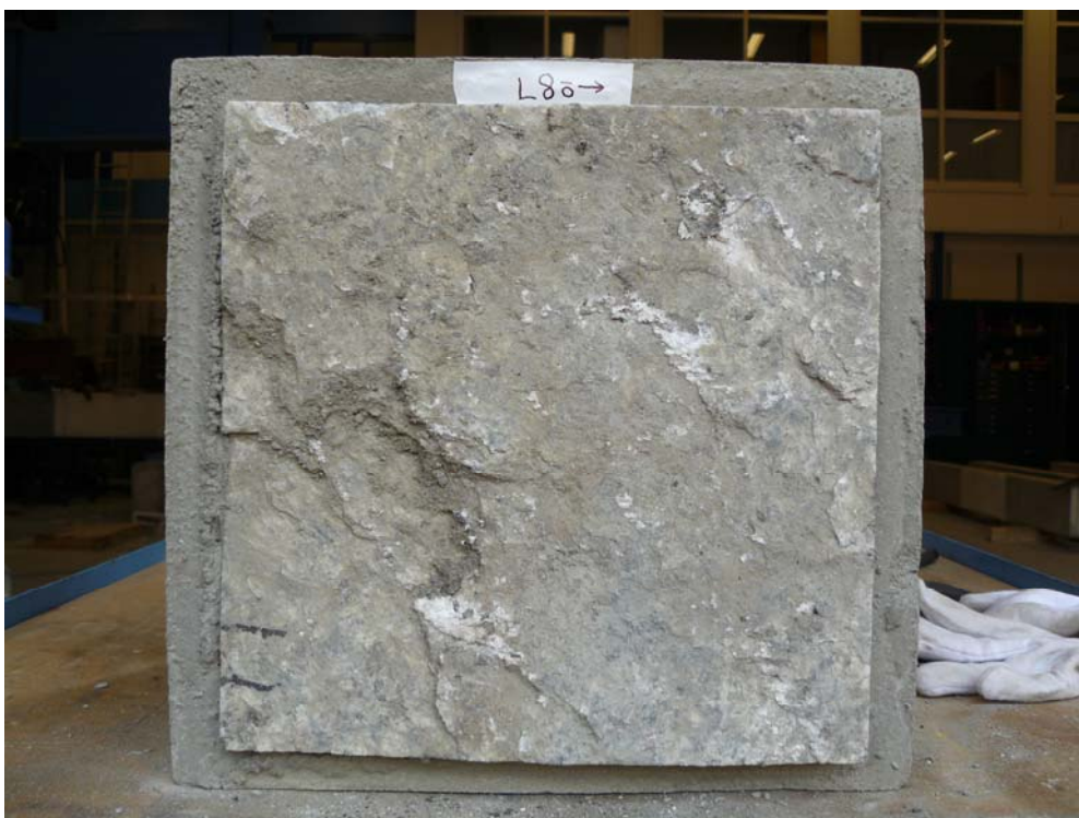
Picture B.12b Sample L9 after the shear test (upper part).
