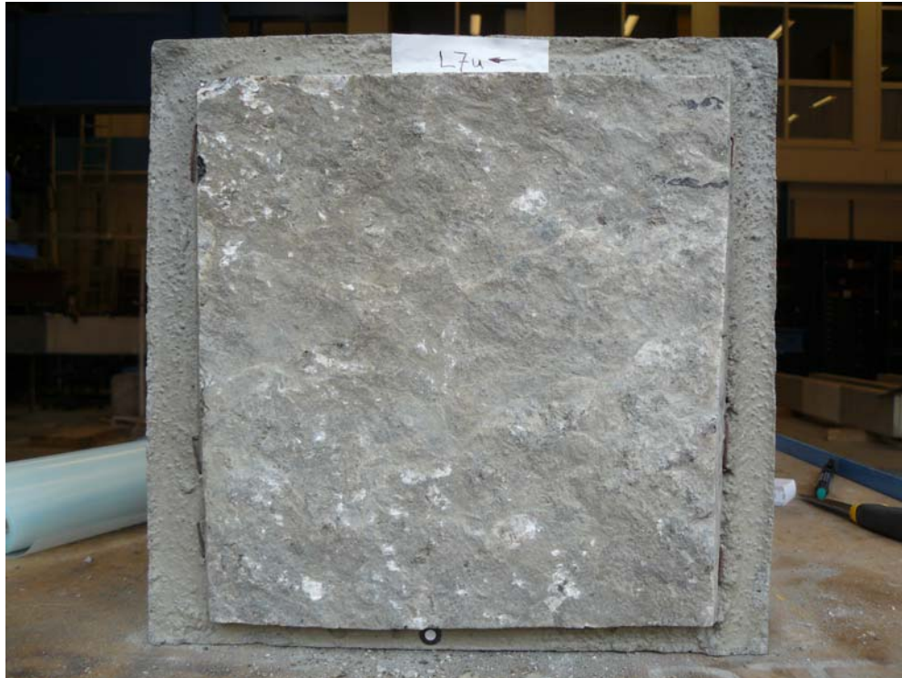
Picture B.11a Sample L7 after the shear test (lower part).
