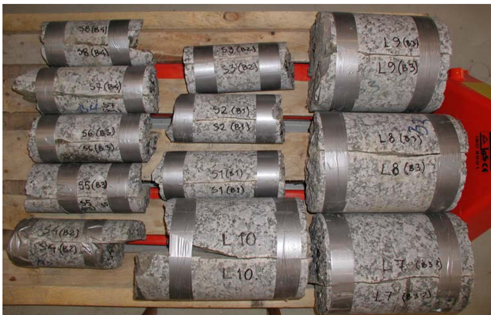
Figure 5.10 Samples sent to LTU for shear testing.
