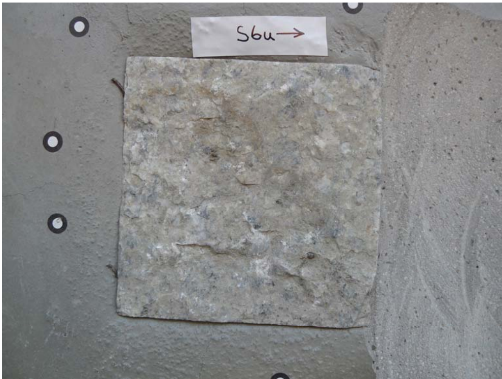
Picture B.6a Sample S6 after the shear test (lower part).
