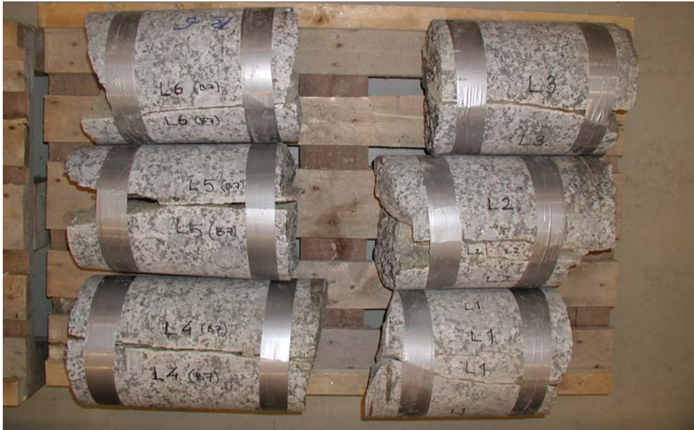
Figure 5.11 Samples sent to LTU for shear testing.
