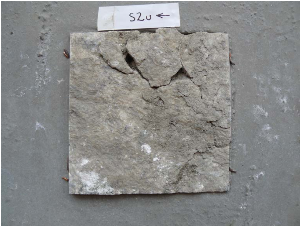
Picture B.2a Sample S2 after the shear test (lower part).
