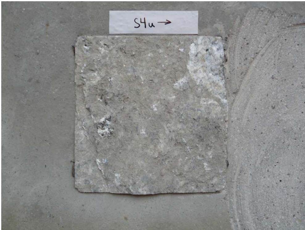
Picture B.4a Sample S4 after the shear test (lower part).
