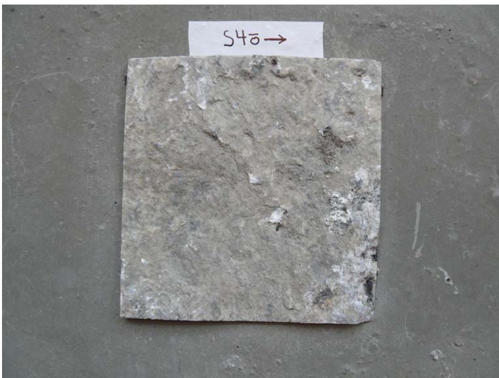
Picture B.4b Sample S4 after the shear test (upper part).
