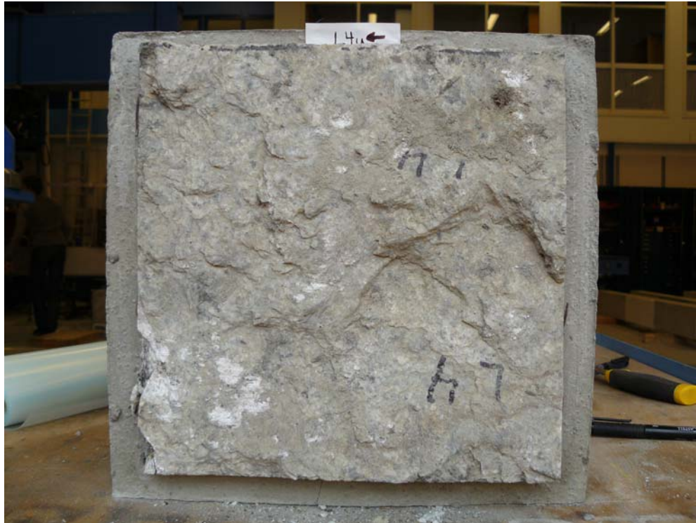
Picture B.9a Sample L4 after the shear test (lower part).
