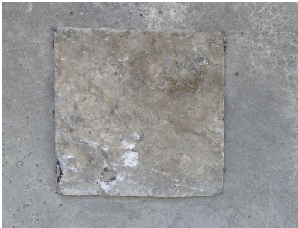
Picture B.7b Sample S8 after the shear test (upper part).
